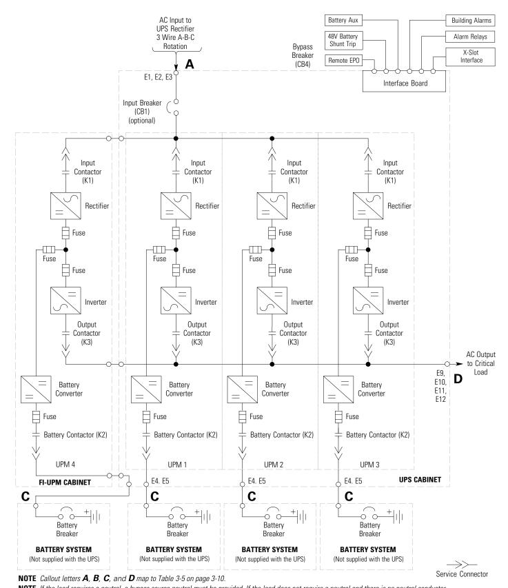
Figure 6-12. Plus 1 UPS System – Common Rectifier Feed, Separate Battery, IOM Configuration
